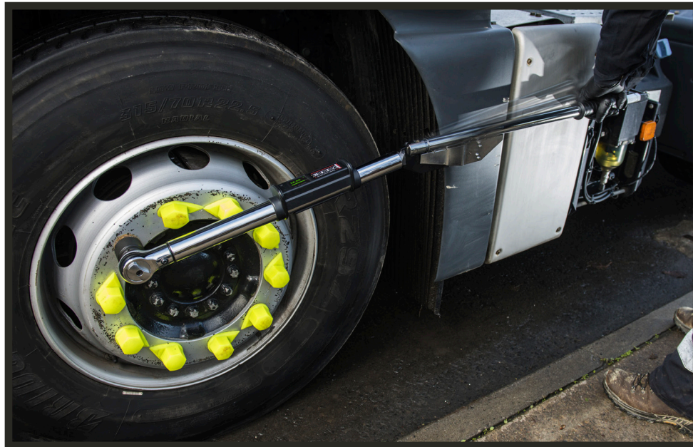
An SB750S breaking over at set torque
